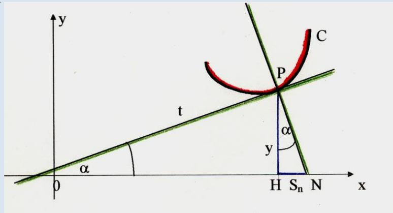
$$\operatorname{tg} \alpha = \frac{HN}{HP} = \frac{S_n}{y} \Rightarrow \operatorname{tg} \alpha = \frac{dy}{dx} \therefore \frac{dy}{dx} = \frac{S_n}{y} \therefore y \cdot \left(\frac{dy}{dx}\right) = S_n \Rightarrow S_n = p \therefore y \cdot \left(\frac{dy}{dx}\right) = p \quad (1)$$
